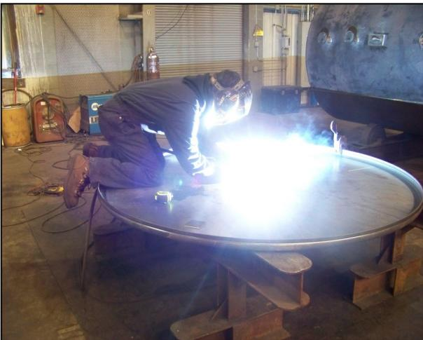
Greer's welding processes include: Submerged Arc Weld (SAW), Flux Cored Arc Welding (FCAW), Gas Metal Arc Welding (GMAW), Gas Tungsten Arc Welding (GTAW), Shielded Metal Arc Welding (SMAW) and Resistance Spot Welding (RSW).
